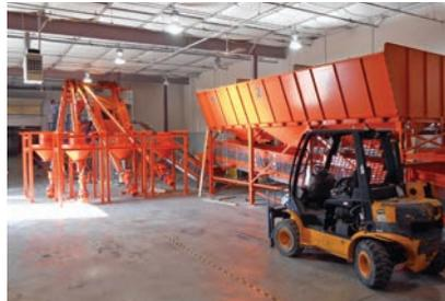
**New concrete batching plant**
